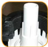
5. Place white gasket over the centre tube before inserting pipe adaptor - ensure fully engaged to produce water tight seal.
