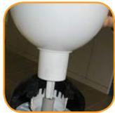
3. Position resin funnel in the distribution pipe. Fill with Resin.
